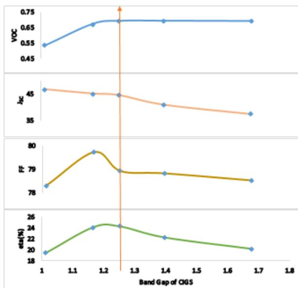
**Fig. 2.** Output of bandgap of CIGS layer change
