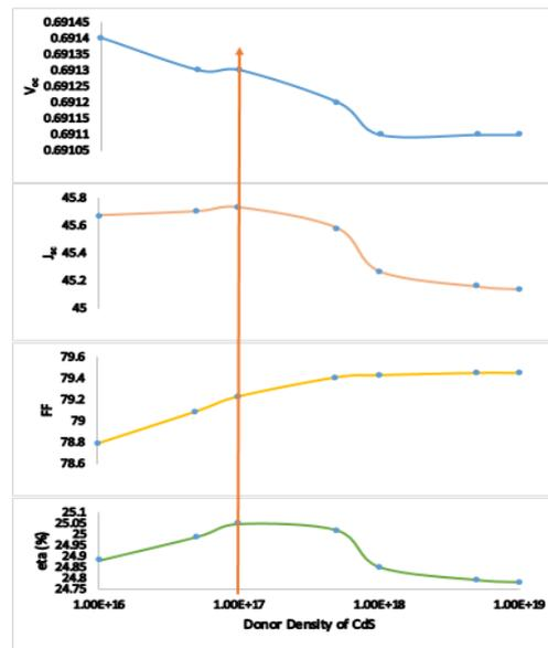
Fig.6. Output of Donor density of CdS layer Change
