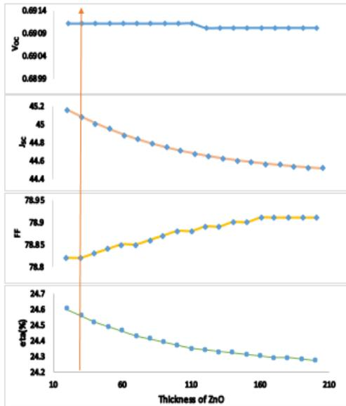
Fig.3. Output of thickness of ZnO layer Change
