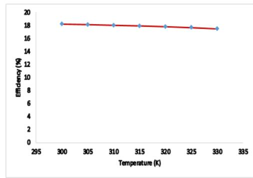
Fig. 14. Temperature vs. efficiency curve of proposed cell
