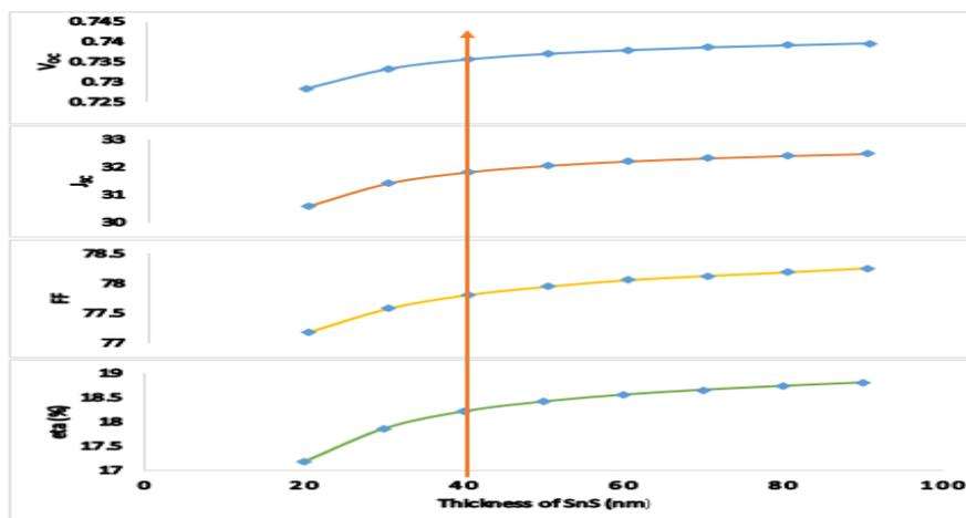
Fig.10. Output of ultra-thin CIGS cell with SnS BSF layer thickness change
