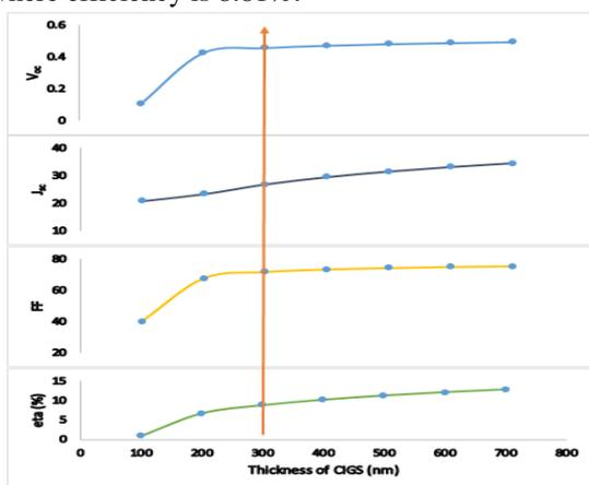
Fig.9. Output of thickness of CIGS layer Change to ultra-thin cell
