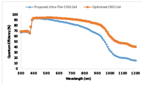
Fig.13. Quantum Efficiency of Proposed cell and Optimized cell
