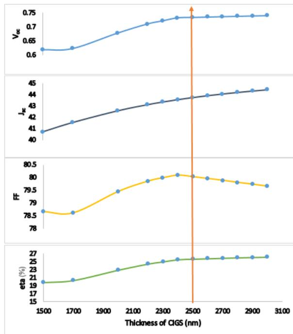
Fig.8. Output of thickness of CIGS layer Change
