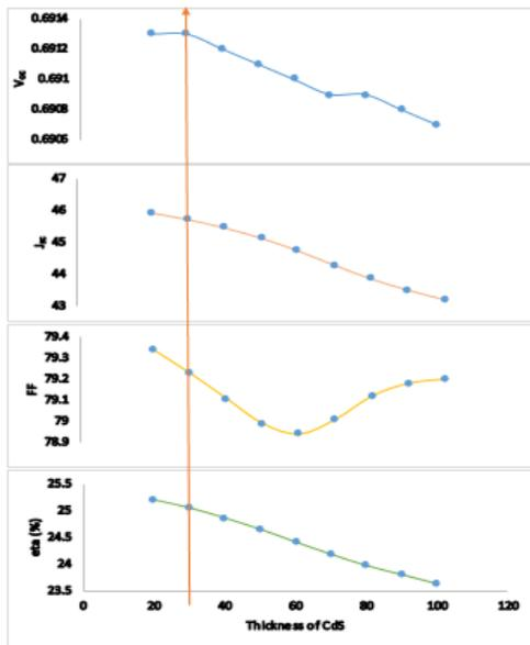
Fig.5. Output of thickness of CdS layer Change
