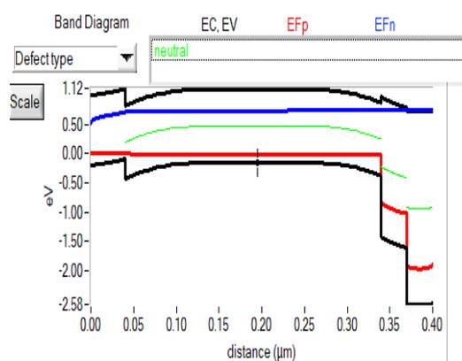
Fig. 12. Band diagram of Proposed cell
