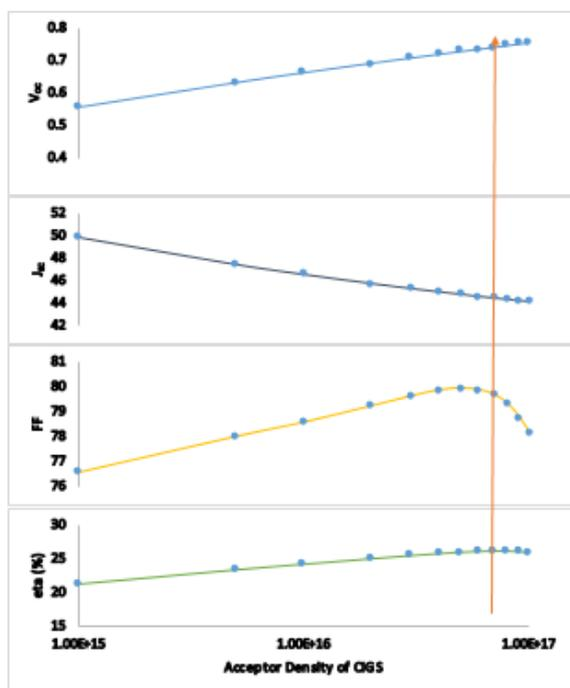
Fig.7. Output of Acceptor density of CIGS layer Change
